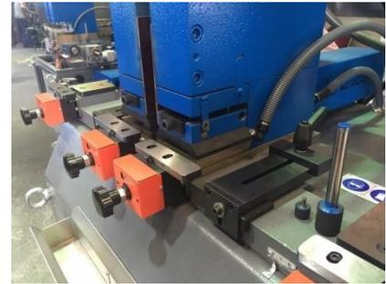
pull out the "Upper Jaw retaining pin"
