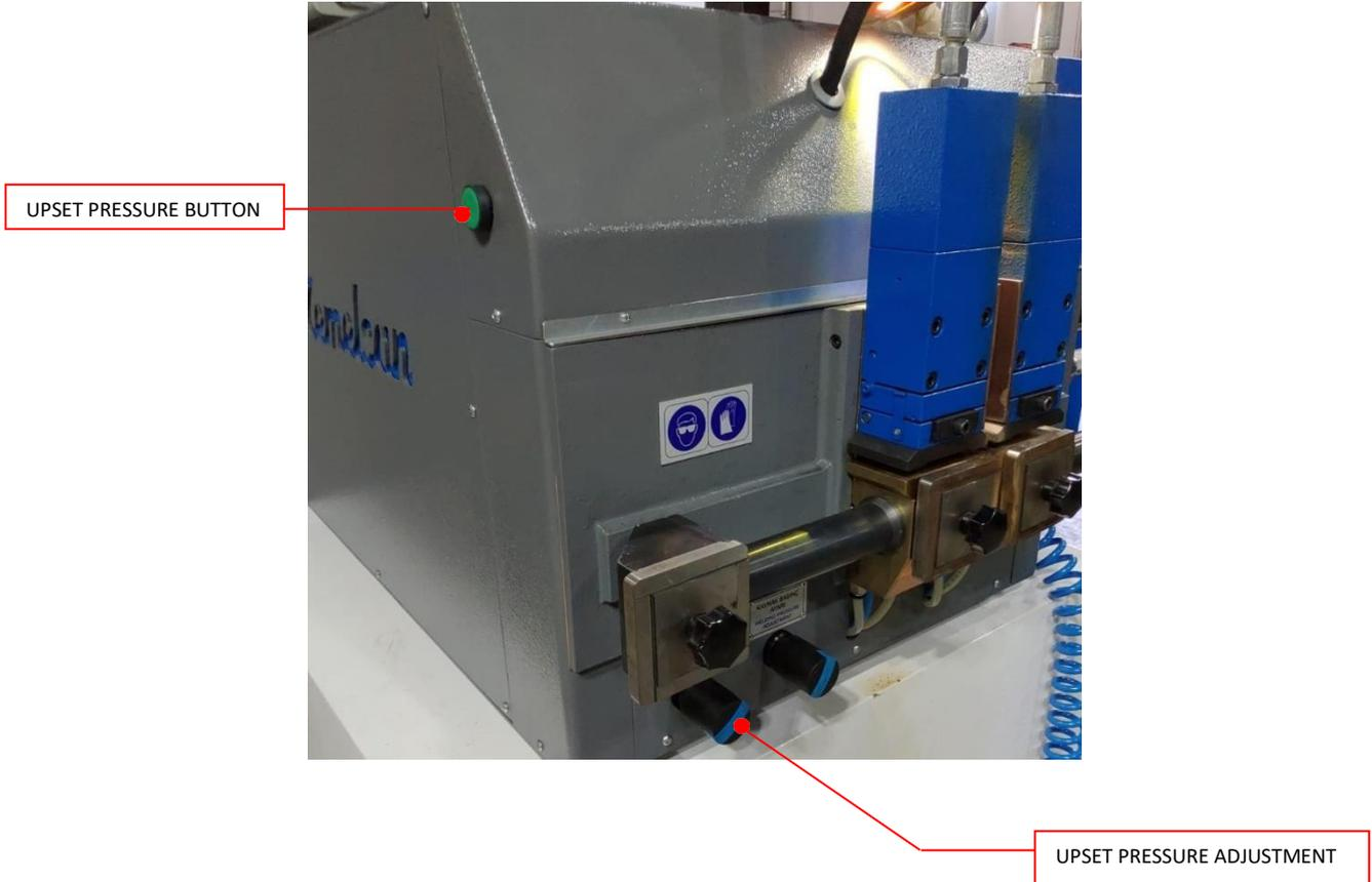
When ones the Welding Ready position is reached by the Clamping Jaws, it's anytime possible to push the Green Button, called Upset Pressure-Button.
