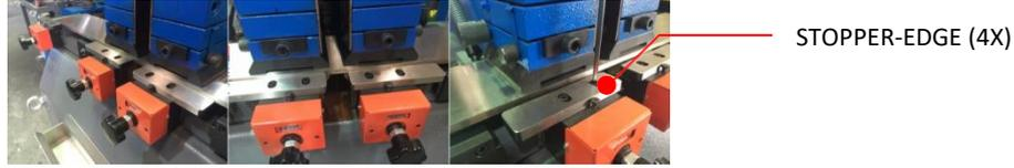
Disengage the all stopper-edges
