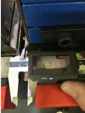
Adjust the space between the Jaws in Welding Ready Position to a specific slot width and measure it proper.
