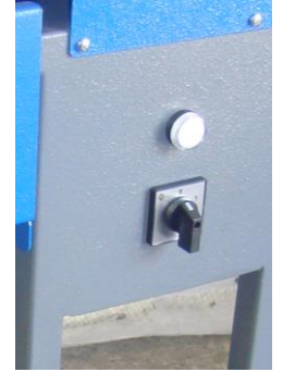
MAIN ON/OFF SWITCH
