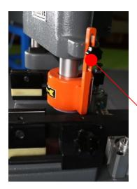
PROTECTION COVER LEVEL ADJUSTMENT SCREWS
