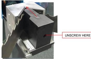
Remove the blade and replace the other dimension that is needed then screw it back
